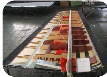
Defective bonding of a fin in a light aircraft wing
